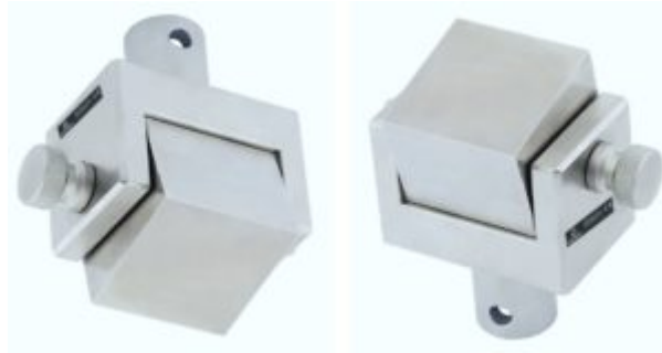
ASTM C297 2" BLOCKS TESTING FIXTURE
