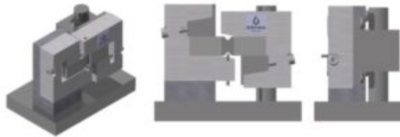
ASTM D5379 Testing Fixture
