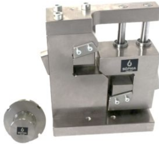
ASTM D 5379 Testing Fixture - Application
