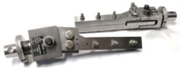
ASTM D 4255-A Testing Fixture - Application
