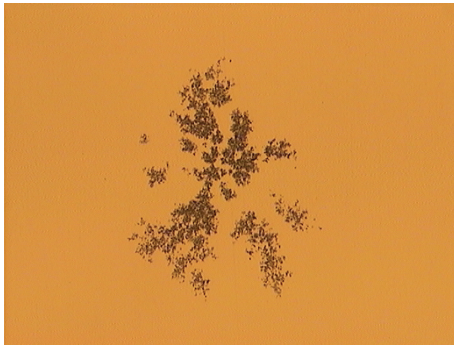
FIGURE 7: 200x magnification of Eta-phase on sample B.
