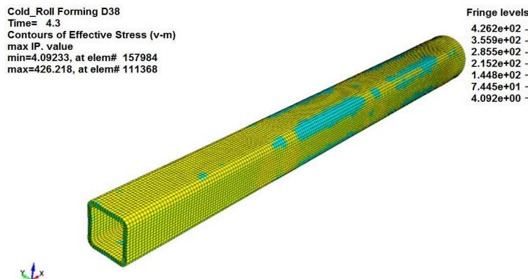
**Fig. 5: Von Mises equivalent stress distribution on the semi-finished product at 4.3 s**
