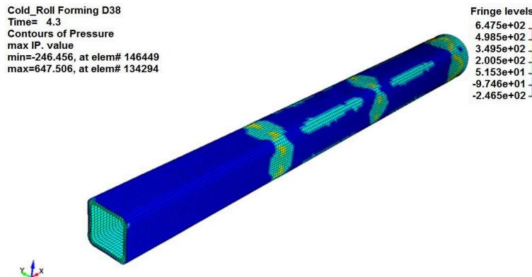
**Fig. 4: Pressure distribution on the semi-finished product at 4.3 s**
