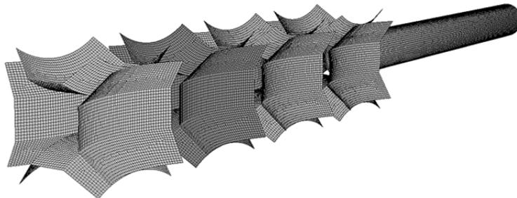
**Fig. 2: FE-Model of the cold roll forming process**
