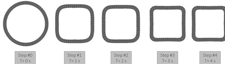
**Fig. 3: FEM analysis on the five advancement stages in the technological process**
