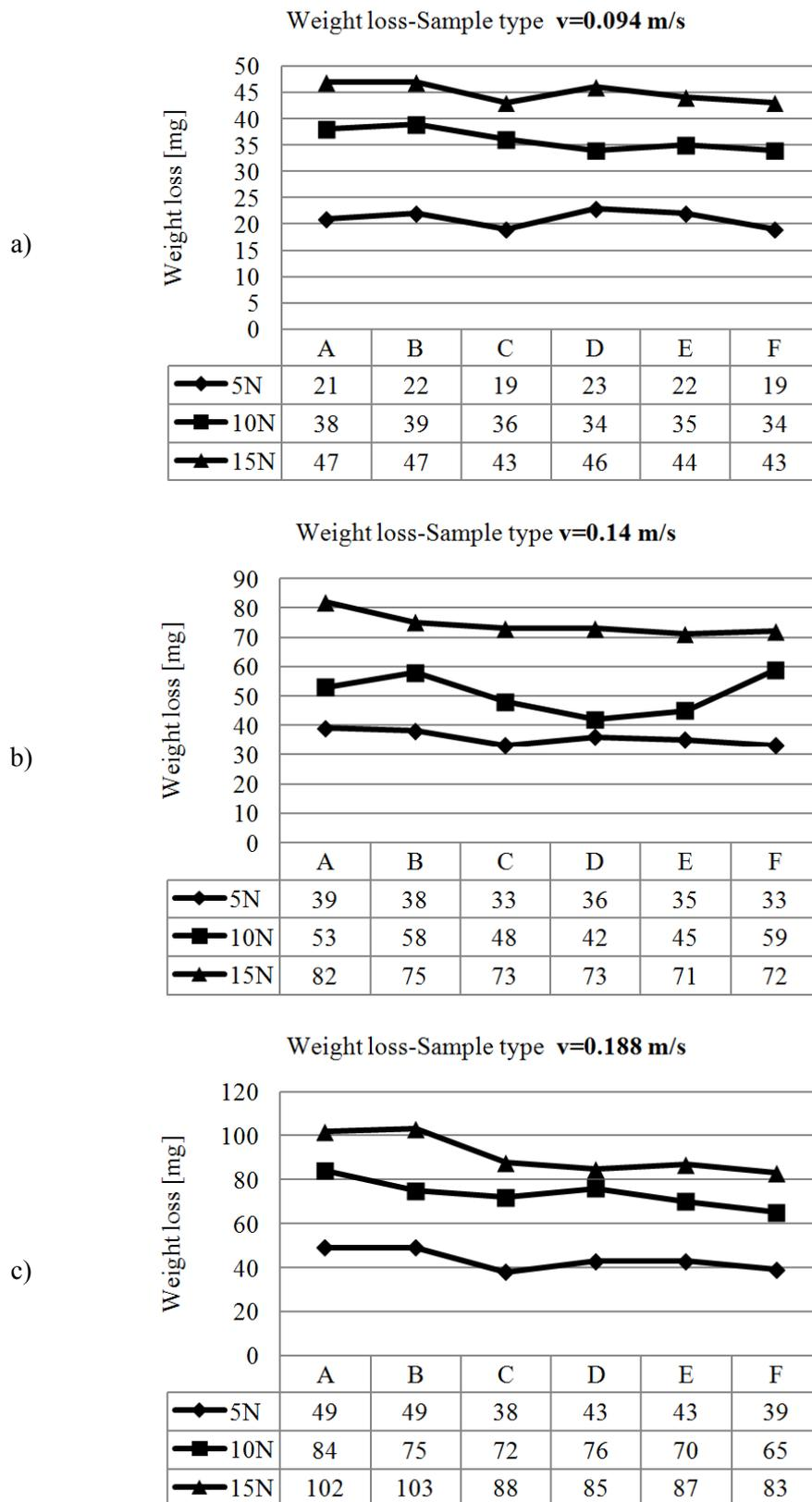
Figure 2: Weight loss for each specimen; tests carried out at speeds of a) 0.094 m/s b) 0.14 m/s c) 0.188 m/s and variable load
