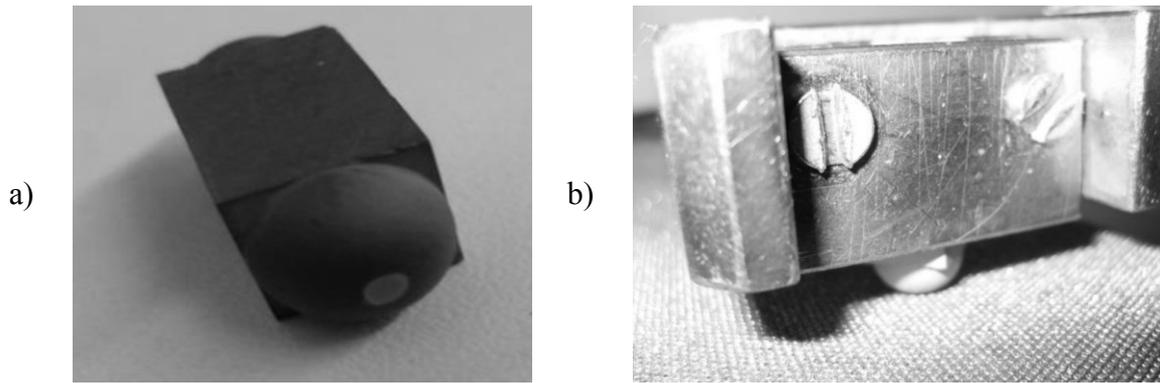
**Figure 1: Sample a) free b) assembled in the pin-on-disk apparatus**
