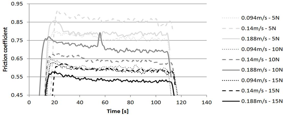
Figure 3: Friction coefficient trend for D sample test
