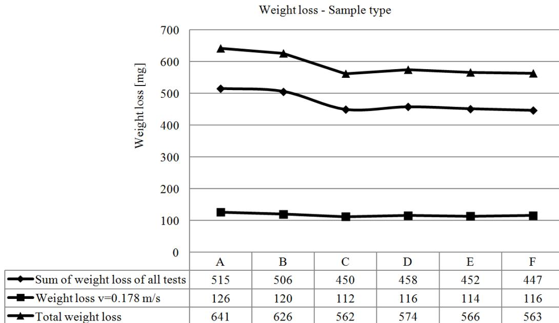
**Figure 5: Weight loss trend @ v=0.178 m/s, Sum of weight loss trend, and total weight loss trend for each specimen after the carried out tests**
