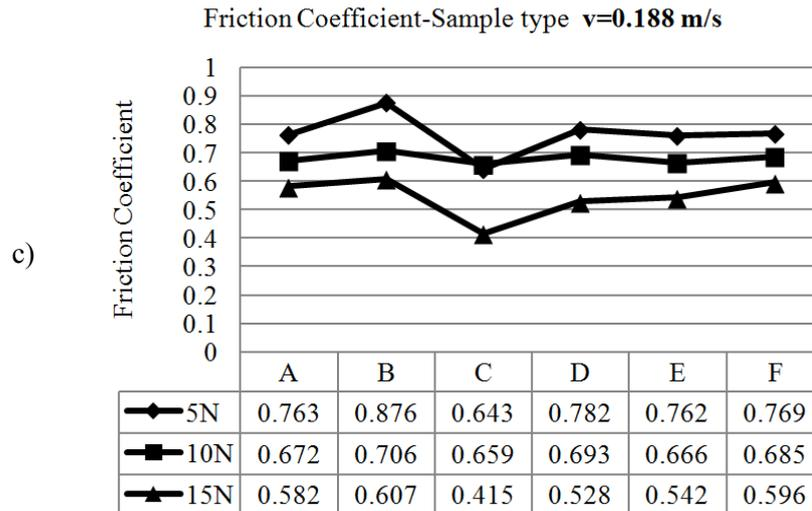
**Figure 4: Friction coefficient for each specimen; tests carried out at speeds of a) 0.094 m/s b) 0.14 m/s c) 0.188 m/s and variable load**
